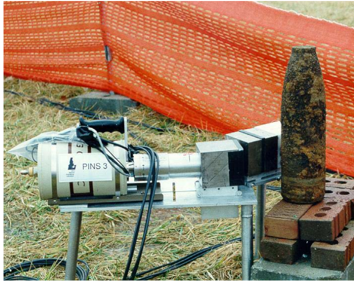
Figure 5. Prompt Gamma Neutron Activation Analysis Setup
